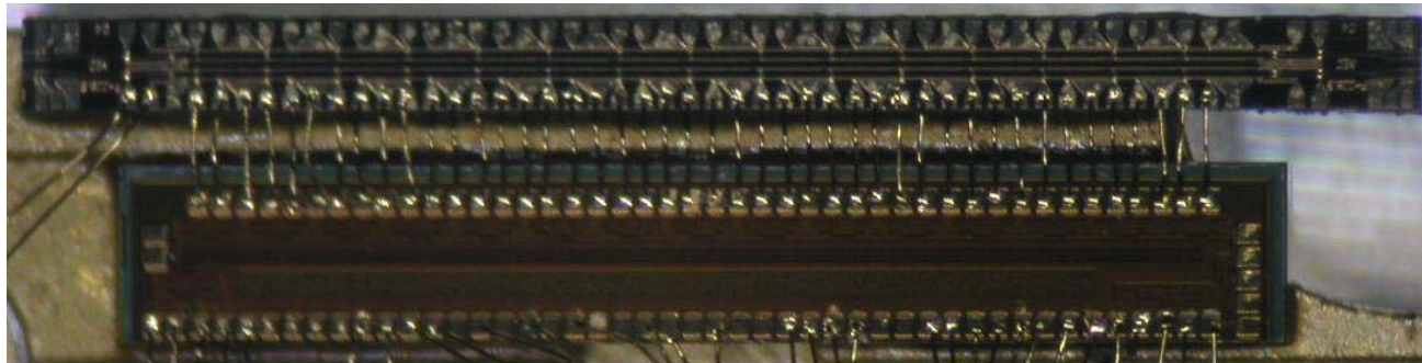
Driver IC (5 mm × 0.9 mm, 90-nm CMOS process)
